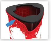
7. Angle and tuck gasket into channel in edge of counter top. Insert graphic gasket all the way around.
